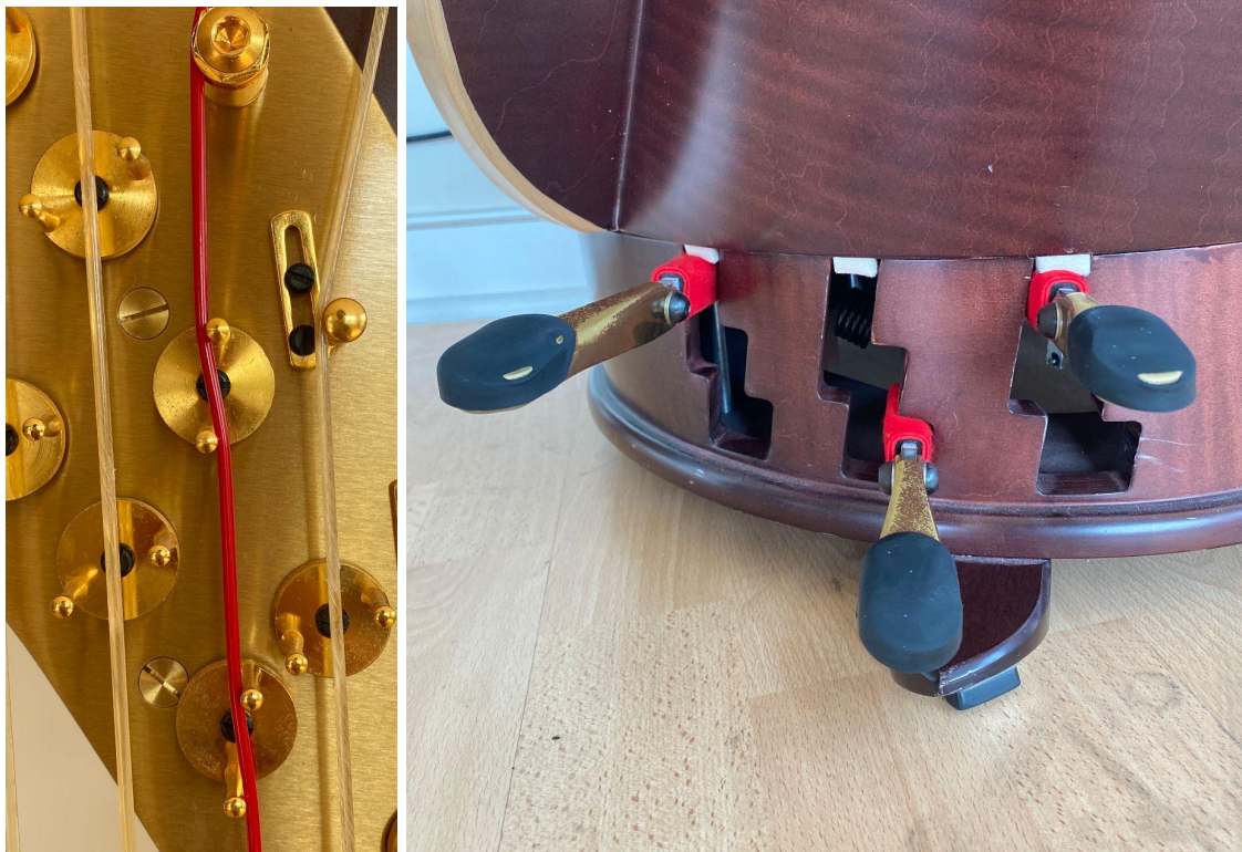
Figure 1.14 - The C pedal engaged in the sharp position (right), turning the first and second discs against the C string and raising the pitch (left.)
