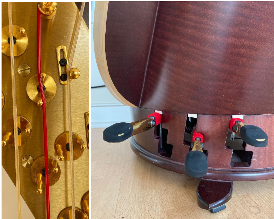
Figure 1.13 - The C pedal engaged in the natural position (right), turning the first disc against the C string and raising the pitch (left.)
